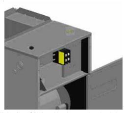
Install the four SPW-01 kit wires to the circuit breaker lugs and torque lug screws to 35 in-lbs. Ensure all wires are tucked inside the control box.
